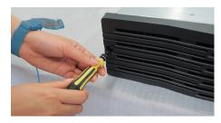
**3.** Align the hard disk with the slot and push in the hard disk gently and steadily.
