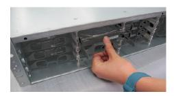
**5.** Cover the front panel and fix the screws to secure the front panel.
